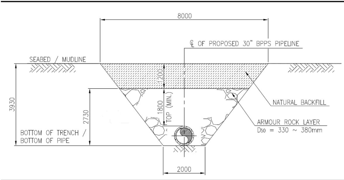
**Figure 3.6 Trench Design (Type F)**
