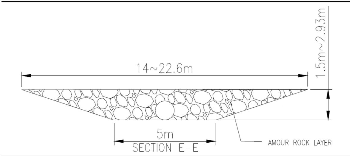
**Figure 3.2 Trench Design (Type B)**
